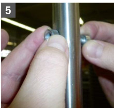
5 Adjust the telescopic rod of the operating pipe, if required with extension for large shaft depths.
