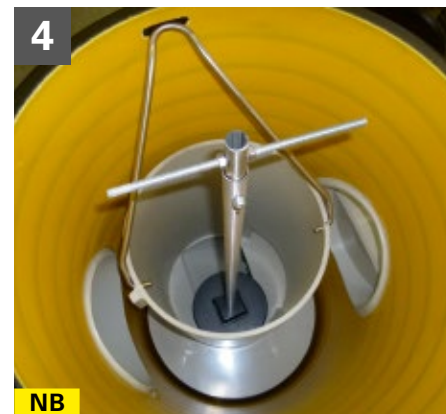
NB The bayonet nut connector is closed if the handles point towards inlet and outlet. Close by turning clockwise.
