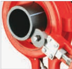
ROCUT® 110 with cutter blade (No. 54950) (special accessories)
