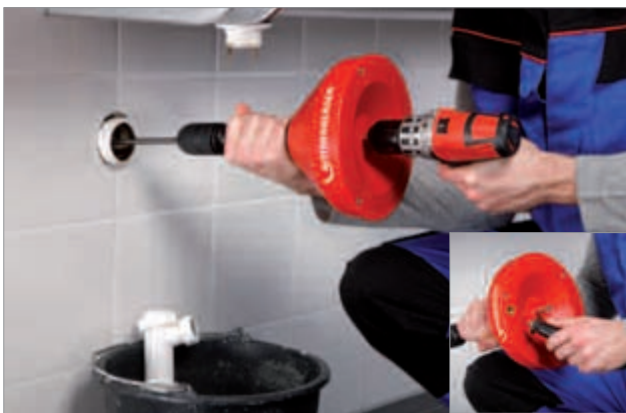
Electrical operation with cordless drill
