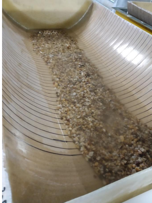
Photo 3 – Test sample filled with gravel/water mixture
