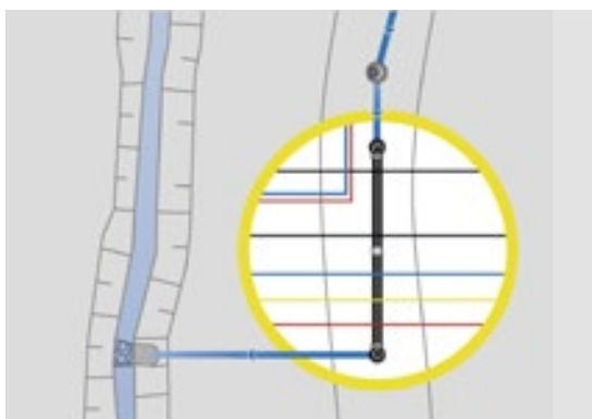
SediPipe XL, integrated into an existing stormwater sewer
