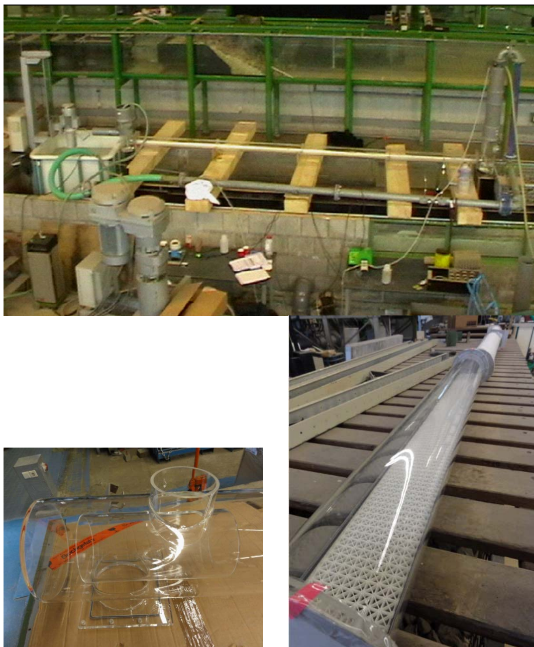
Figure 1.4: The SediPipe scaled model in the lab of TU Delft
