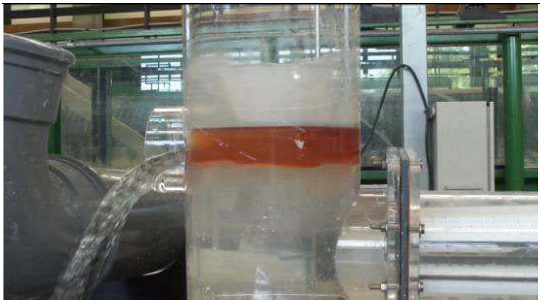
Figure 2.5: No flush out of oil
